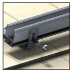
7. Attach the rail to the tile using 3/8" bolts, washer & nut. (Recommended: place star washer between the rail & flat tile hook).
