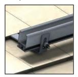
8. Secure the 3/8" bolt with the nut. (Tightening torque 14 ft-lbs).
