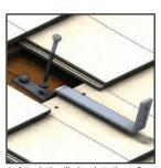
4. Attach the tile hook to the rafter using the two 3/16" or 5/16" lag bolts, embedded min. 2.5". Tighten carefully.
