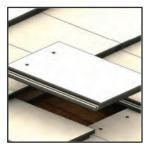
1. Remove the roof tile at the marked position or, if possible simply push it up.
